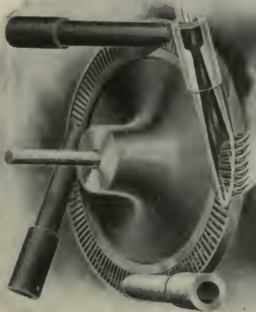
A TURBINE WHEEL AND ITS NOZZLES Showing how the steam is applied directly to a revolving disc.
